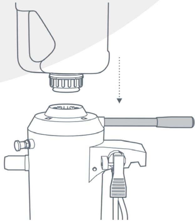
**A container with an easyconnect cap is connected to the coupler.**
