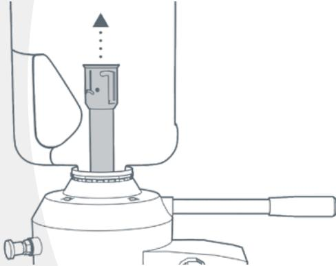
To empty the container, the coupler probe pushes the internal connecting plug of the easyconnect cap into the container, thereby allowing the liquid contents to be emptied via the coupler into the tank.
