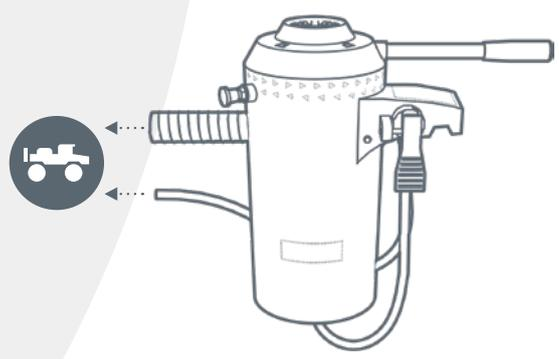
The coupler connects to a sprayer tank to transfer the product into the sprayer.
